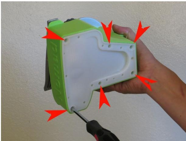
6. With all six screws removed the water tank can be removed from the case. The water tank fill spout fits tight inside a sealing O-Ring. To remove the tank grasp the green case and push down on the water tank white fill spout.
