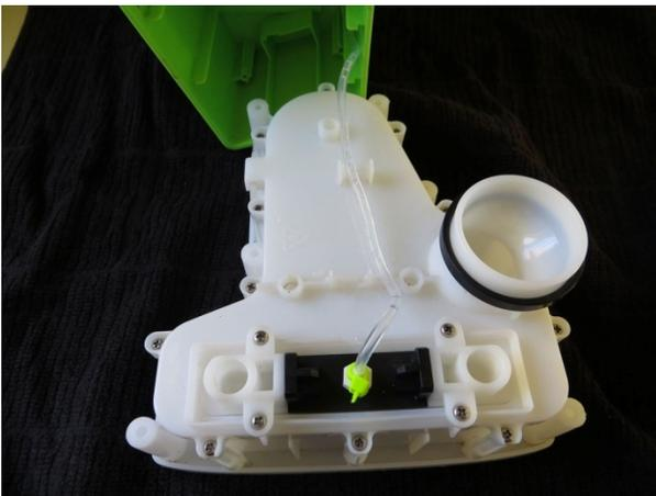
8. Remove the four screws holding the pump.
