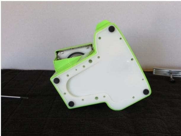
5. Using a long Phillips screwdriver remove the six screws holding the water tank to the case.
