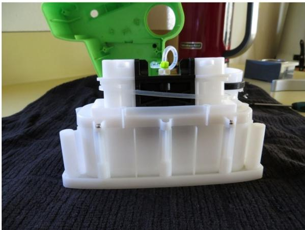
10. At the bottom of the pump where the old umbrella valve stem protrudes out of the bottom edge use diagonal cutters or a sharp knife to cut off the stem flush with the bottom. Use a small tool to push the valve up into the cylinder and a long small screwdriver to "fish" it out of the cylinder.
