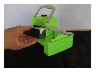
3. Remove the two screws from the drawer latch lever and lift the latch lever off.
