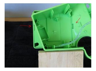
6. This tab can be released from the top by sliding a small long flat screwdriver or other flat blade object between the cube edge and case edge as in the image below. The blade must stay low and go to the midpoint of the cube case. When it releases you will hear a click or pop as it opens. (While this image shows the latch lever on in reality yours should be removed at this point).
