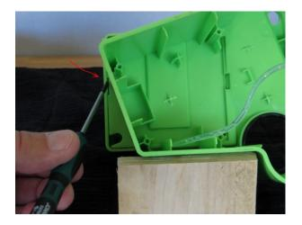
5. The other tab is directly opposite the first tab, its location is shown in this open case image below. <u>This view</u> is shown for clarity, it is not necessary to open the case to remove the cube cover.
