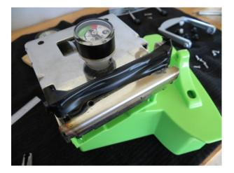
9. Now you can use the open end wrench to remove the old gauge. Inspect the gauge hole to make sure it is free of debris.
