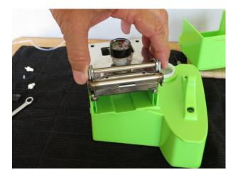
12. Make sure the white tension washer and arms are as in the image below. (Notice the dish direction of the white tension washer)
